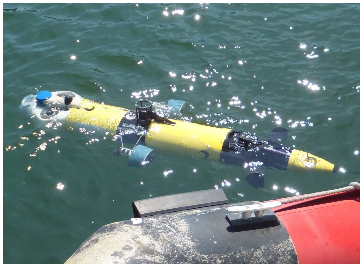
Figure 10: VAMA (Véhicule Anti Mine Autonome), an AUV owned by DGA Tn.
