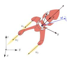
The inertia matrix  $\mathbf{I}$ , the mass m are assumed to be constant. The state is composed of
