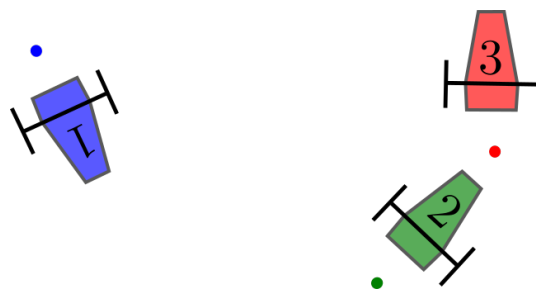
Figure 5.3: R_1 follows R_2 , R_2 follows R_3 , R_3 follows R_1 . The artificial hooks are represented by the points at the back of each vehicle
