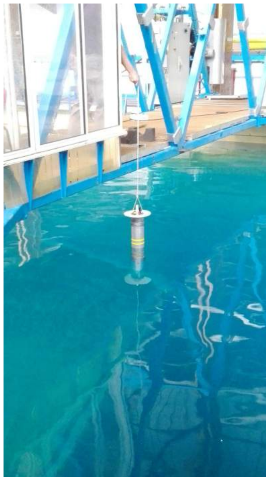
Figure 3.13: Deployment of the Ifremer float in the pool with a line
