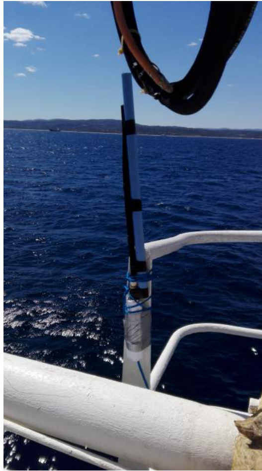
Figure 3.10: Bullet antenna attached to the ship
