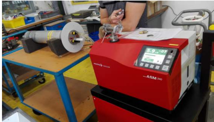
Figure 4.25: Installation of the mass spectrometer to detect the leak in the float
