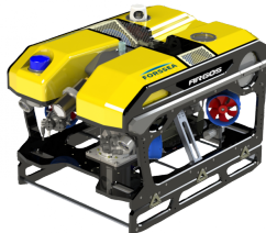
(a) ARGOS - Hybrid Light-Intervention Smart ROV
