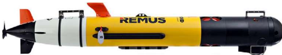
Figure 4: Remus100 : Actuated in surge, pitch and yaw, used on task requiring 3 translations (Credit: WOI)
