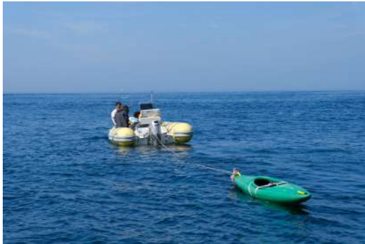
Boatbot towing a magnetometer
