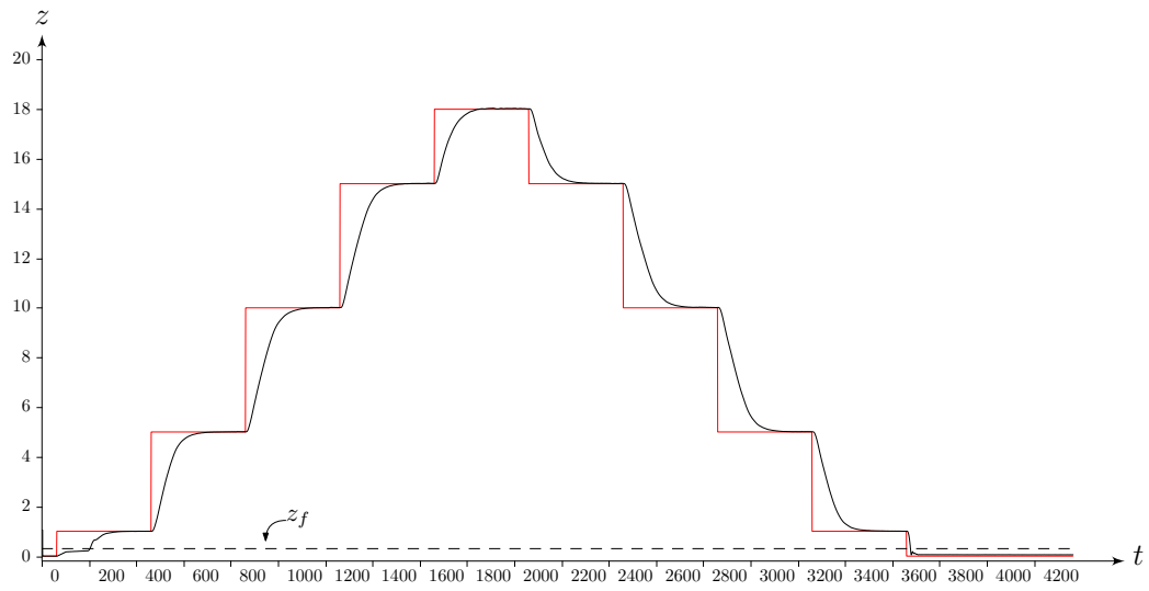
Figure 5.13: Depth z (in meter) of the float in function of time t (in seconds). The setpoint depth trajectory is in red and the float depth trajectory is in black.
