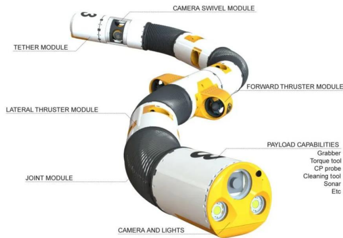
Figure 6 Eelume design and components [17]
