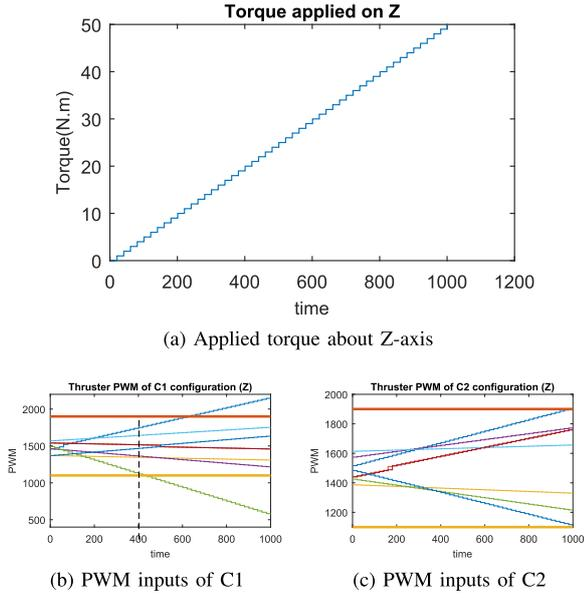
Fig. 11: The simulation of cube rotation about Z-axis for  $C^1$  and  $C^2$
