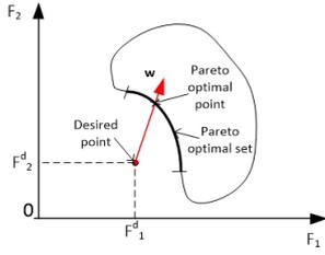
Fig. 5: Goal attainment method with two objective functions
