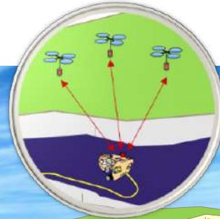
Magnetic Positioning System using Aerial Drones
